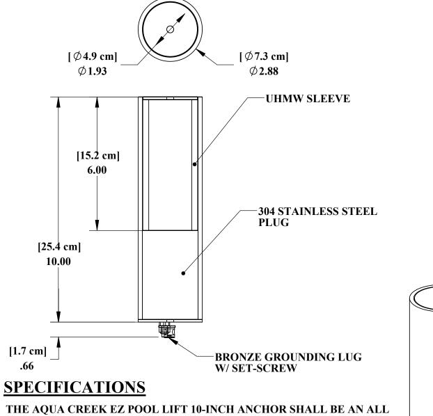
STAINLESS STEEL ANCHOR WITH A UHMW PIVOT SLEEVE. THE ANCHOR SHALL FIT A 1.90" [4.8 cm] O.D. MAST. THE ANCHOR SHALL COME STANDARD WITH A BRONZÉ GROUNDING LUG ATTACHED AT THE BOTTOM, AND AN ELECTRO-POLISHED TAMPER RESISTANT LID.
